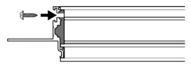
5. Firmly attach the nail fin to the window frame with contractor supplied 5/8" self tapping screws in the pre-drilled holes through the nail fin. Warning - 5/8" screw length are critical to installation.
