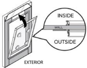
2. Lift the **window frame** into the rough opening. From nail fin, to face of INICIO frame is approximately 1". This is the exterior of the INICIO window.
