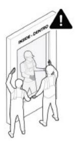
2. Make sure the **window frame** is held in position for the rest of the installation.
