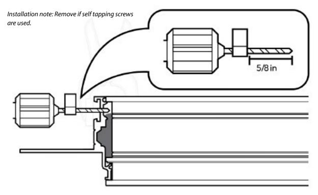
4. Mark a 1/8 - inch drill bit at 5/8 inches with tape, and drill holes spaced 12 inches into the side of the nail fin. Make sure to not go too deep or you could cause damage to the frame.
