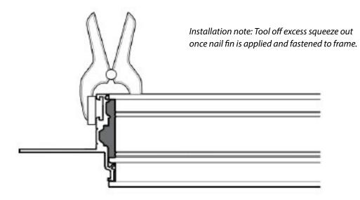
3. Attach the **nail fins** to the **window frame** using clamps.
