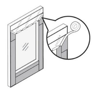
4. Attach the flap onto the flashing using home wrap tape. Tape the diagonal cuts and the bottom of the flap to the nail fin.
