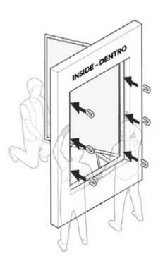
6. Make sure the window frame stays centered by putting plastic horseshoe shims between the jambs and the sides of the **window frame** .
