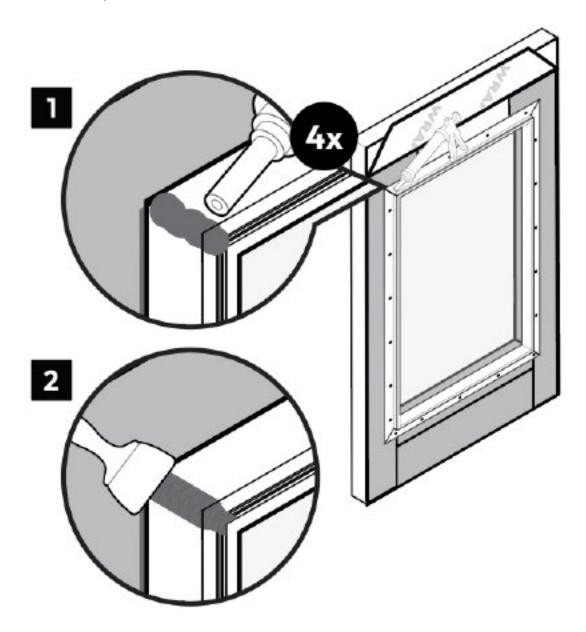
1. Apply sealant on the miters where the **nail fins** meet.
