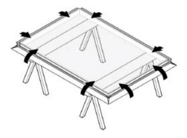
2. Dry - fit all the nail fins to the related side of the window frame, to make sure they fit correctly.
