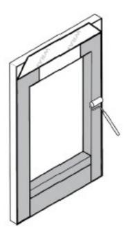
6. Use a J - roller to firmly press all the flashing onto the wall.
