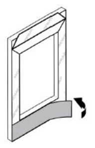
Installation note: Typically use a 9" wide roll of S.A.F. for new construction installations. Bottom apron per Illustration #1 to be used if no WRB (Weather Resistant Barrier) is installed. Skip this step if W.R.B. is in place.
