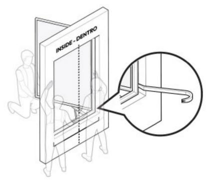
4. Center the **window frame** by moving the **window frame** side-to-side using a prybar. Visually check the sash reveals.
