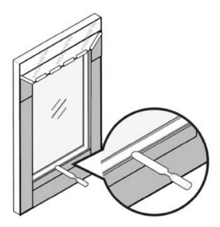
5. Tool the silicone sealant using a spatula, make sure the silicone sealant continuously fills the gap between the window frame and the rough opening.
