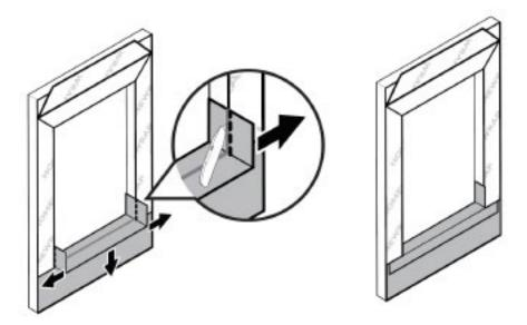
2. Create a flexible sil pan, apply flashing to the base of the rough opening, make cuts in the corners, and fold the flaps over the corners of the rough opening.
