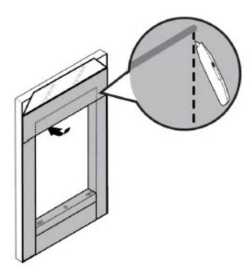
2. Cut the flashing in the corners and fold the flashing into the rough opening. Make sure the entire header is covered by flashing.
