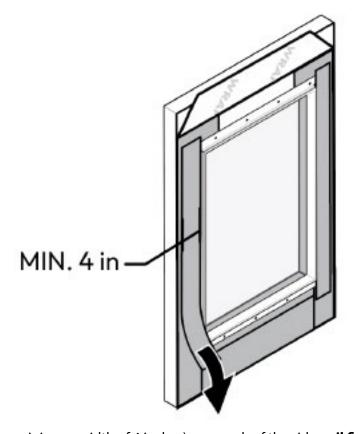
1. Apply flashing (with a minimum width of 4 inches) over each of the side **nail fins** .
