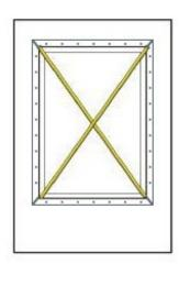
7. Check if the diagonal measurements of the window frame are equal to check for square. Adjust as necessary to where diagonal measurements are exactly equal.
