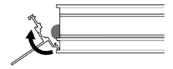
2. Tilt the **nail fin** into the side of the **window frame** . Make sure the bead of sealant on the **middle lip** is pressed between the **nail fin** and the **window frame** .
