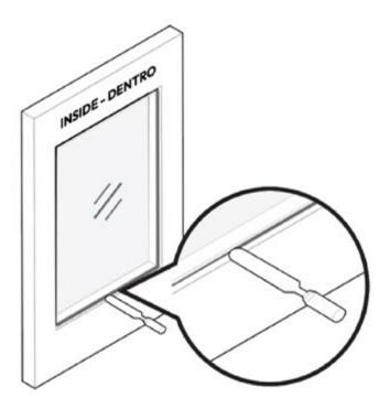
1. Push a backer rod into the gap around the whole perimeter between the **window frame** and the rough opening.
