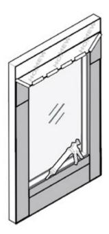
4. Fill the gap between the **window frame** and the rough opening with silicone sealant.
