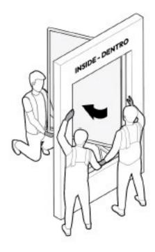
3. Open the window all the way. Make sure the **sash** is supported.
