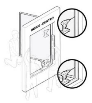
7. Attach the **window fram**e to the jambs by driving the provided **truss head screws** into the upper and lower corners of the **window frame**.
