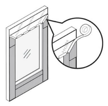
2. Attach the flap onto the flashing using home wrap tape. Tape the diagonal cuts and the bottom of the flap to the header.
