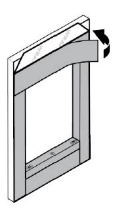
1. Apply a strip of flashing to the header.
