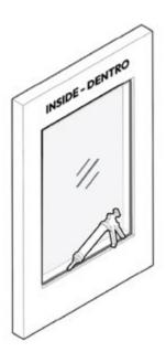
2. Fill the gap between the **window frame** and the rough opening with silicone sealant.
