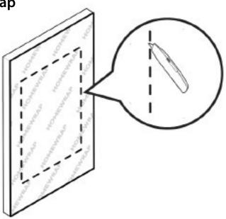
1. Cut an opening in the home wrap matching the dimensions of the rough opening where the window is installed.
