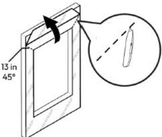
2. Make 13- inch long, 45 - degree diagonal cuts in the upper corners of the home wrap. Tape the cut flap of the home wrap upwards for temporary clearance.
