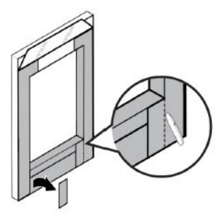
5. Cut away the pieces of flashing directly beneath the lower edge of the window opening. Remove the release paper left on in step 3, and attach the butyl flashing to the flashing underneath.
