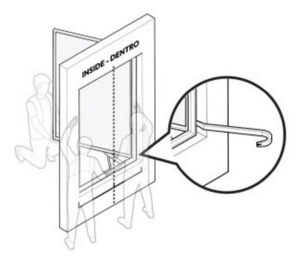
5. Center the **window frame** by moving the **window frame** side- to- side using a prybar. Visually check the sash reveals and adjust where necessary.
