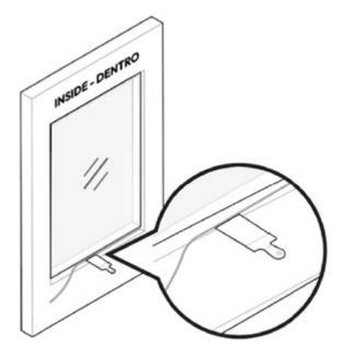
3. Push a backer rod into the gap around the whole perimeter between the **window frame** and the rough opening.
