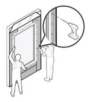
11. Attach the **nail fins** and the **window frame** to the window opening with screws. The manufacturer recommends using 10x3"t screws.
