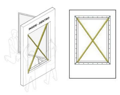
8. Check if the diagonal measurements of the window frame are equal to check for square. Adjust as necessary to where diagonal measurements are exactly equal. Once confirmed, drive screws secure confirming that the frame remains fully square.
