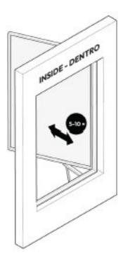
9. Open and close the window for 4–5 cycles to make sure the operation is smooth, and the locks engage fully.
