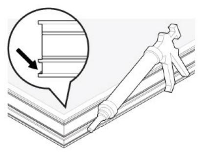
1. Apply a 1/4 - inch bead of silicone sealant on the **bottom lip** around the entire perimeter of the **window frame** using a caulk gun.
