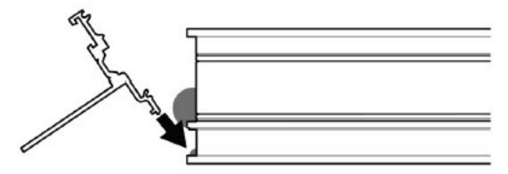
1. Put the bottom of the **nail fin** into the bead of sealant on the **bottom lip**.
