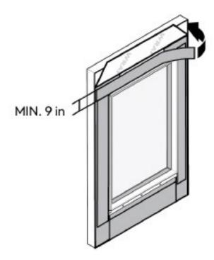
2. Apply flashing (with a minimum width of 9 inches) over the top **nail fin** .
