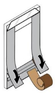
3. Apply flashing along the sides of the window opening, ensuring overlap with the rough opening.
