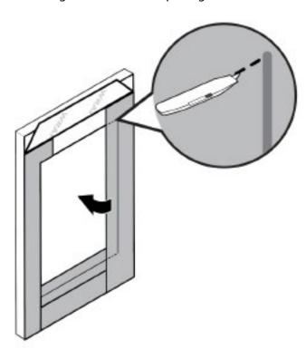
4. Cut the flashing in the corners and fold the flashing into the rough opening. Make sure the entire jamb is covered by flashing.
