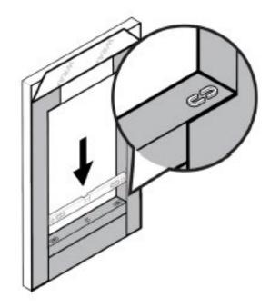
7. Level the rough opening's sill using a level and plastic horseshoe shims
