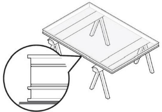
1. Put the **window frame** on saw horses. Make sure the window frame is supported on the aluminum frame and oriented correctly.
