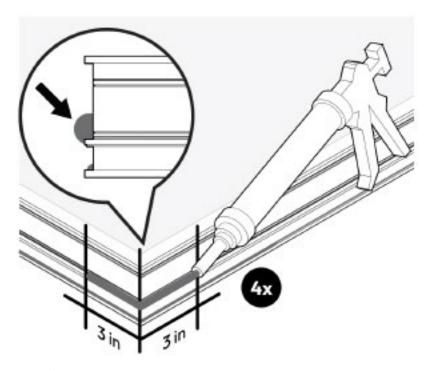
2. Apply a 1- inch bead of silicone sealant on the **middle lip** 3 inches across each **corner** using a caulk gun.
