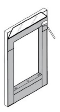
3. Use a J - roller to firmly press the flashing onto the wall.
