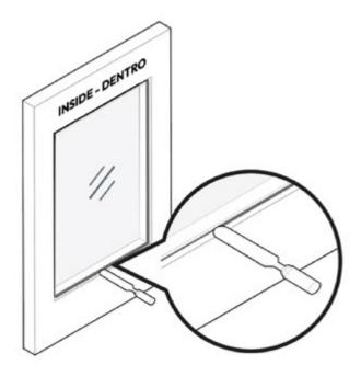
3. Tool the silicone sealant using a spatula, make sure the silicone sealant continuously fills the gap between the window frame and the rough opening.
