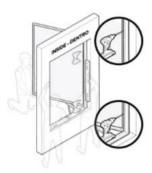
6. Attach the **window frame** to the jambs by driving the provided **truss head screws** into the upper and lower corners of the **window frame**.
