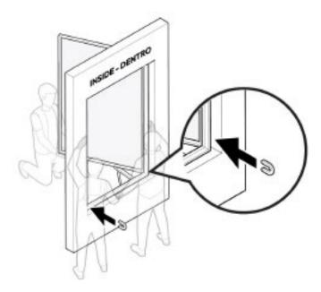
5. Make sure the window frame stays centered by putting plastic horseshoe shims between the jambs and the sides of the **window frame**.
