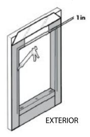
1. Apply a 3/8 - inch bead of silicone sealant 1 inch from the edge of the opening on both sides and top of the rough opening.
