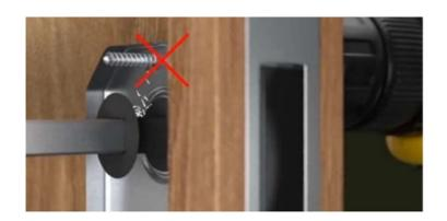
BEFORE DRILLING THROUGH FOR THE HANDLE'S THROUGH-HOLE SCREWS, THE LOCK MUST BE DISMANTLED; OTHERWISE, THERE IS A RISK OF DRILLING THROUGH THE LOCK CASE AND CONTAMINATING THE INTERNAL PARTS WITH METAL FILINGS OR WOOD SHAVINGS, WHICH WILL RESULT IN THE LOCK BEING JAMMED.
