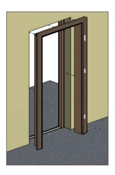
6. SECURE THE DOOR FRAME USING SHIMS AND ADJUSTABLE STRUTS IN THE SPECIFIED ORDER.
